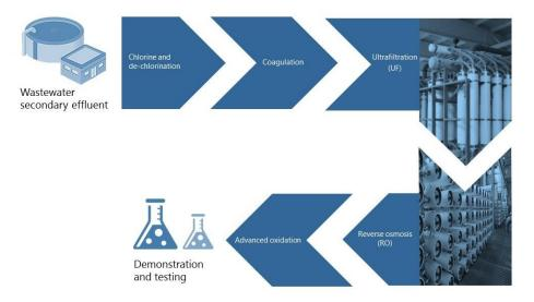
Biwater will provide a complete turnkey design, and supply and commission all process, mechanical, electrical and control components for the plant.
